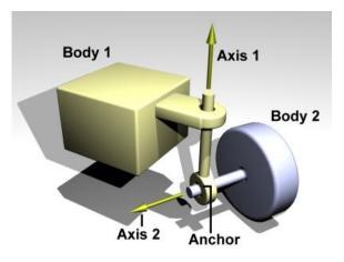
Figure 7.5: A hinge-2 joint.
