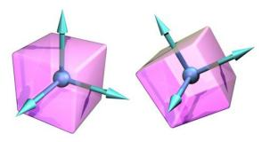
Figure 3.1: The body coordinate frame.
