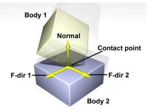
Figure 7.6: A contact joint.
