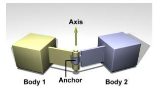
Figure 7.2: A hinge joint.
