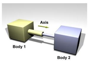
Figure 7.3: A slider joint.
