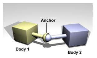
Figure 7.1: A ball and socket joint.
