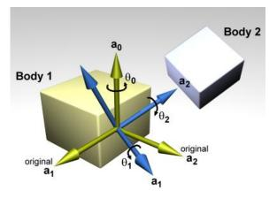
Figure 7.7: An AMotor joint with euler angles.
